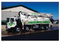
Autocar custom-engineered the chassis for Wm. L. Robinson Concrete's new 45-meter CIFA pump to avoid the need for load permits.
